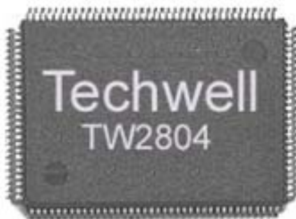
TW2804 128-pin PQFP package
